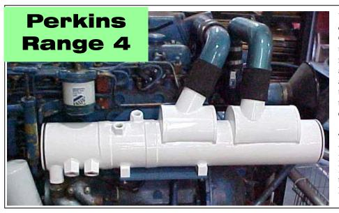
Utilizing a newly designed laser cut custom bracket, this unique Orca Marine Cooling Systems unit mounts neatly on the engine, replacing the entire original 3-part assembly. All hose connections are matched in location, and the unit extends only two inches more than the original, still inside the engine envelope.
